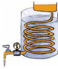
Figure 5. Diagram of the operating principle in case of cylinder and a coil whose juice circulates inside the coil and hot water outside.
